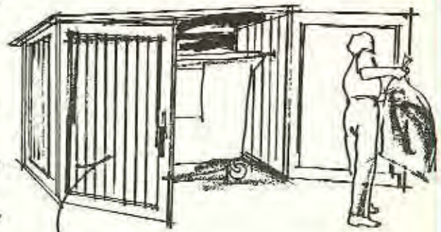
NEW, LOCKABLE DUMPSTER ENCLOSURE, PAINTED OR STAINED
