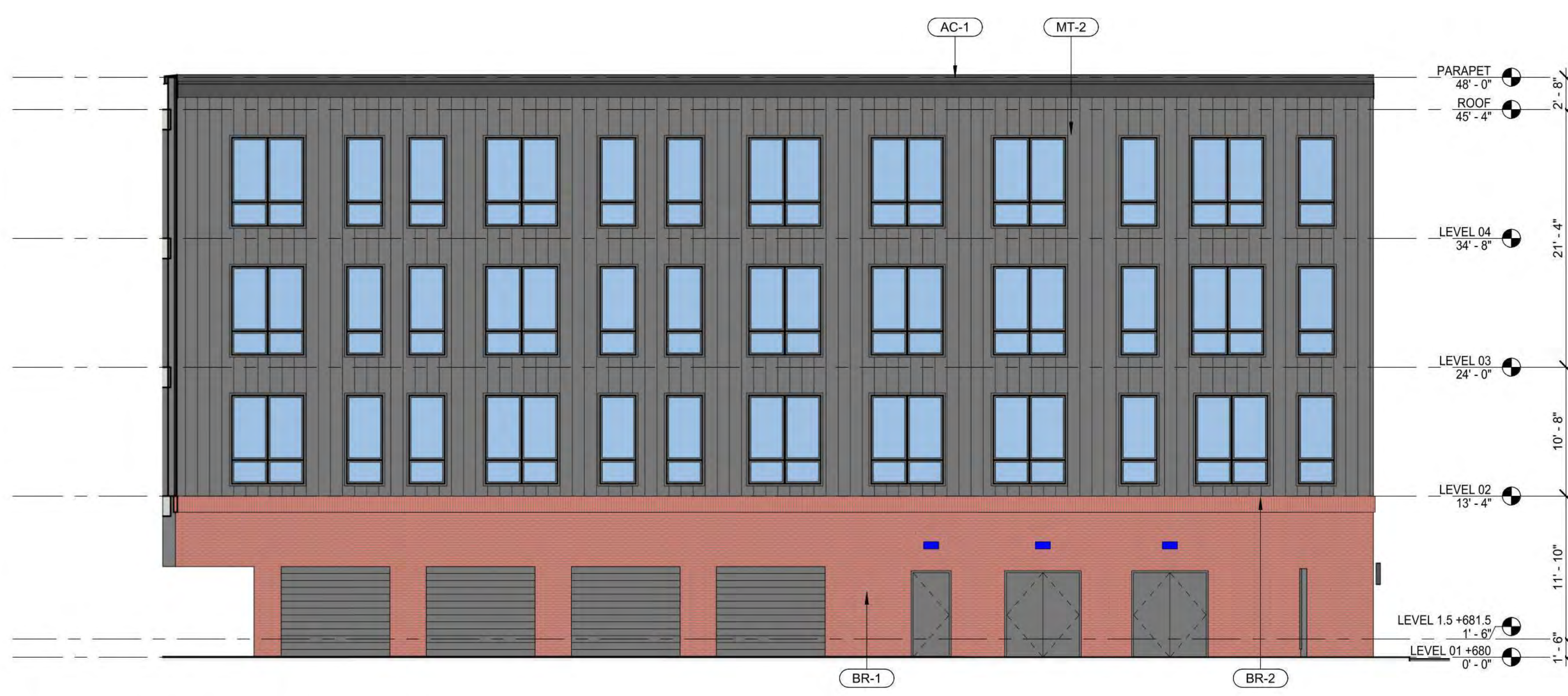
6 BUILDING NORTH - NORTH ELEVATION SCALE: 1/8" = 1'-0"
