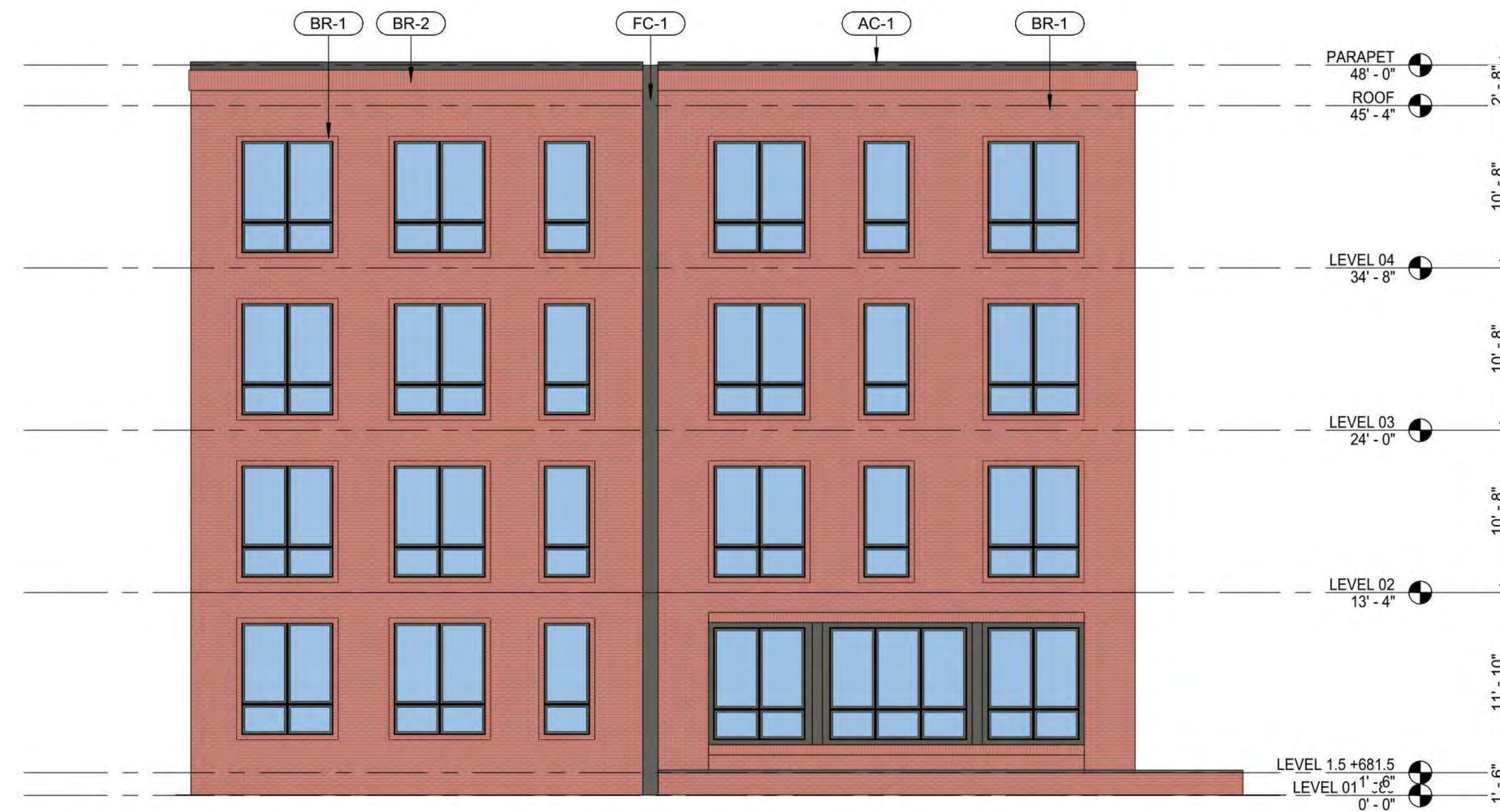
3 BUILDING SOUTH - WEST ELEVATION SCALE: 1/8" = 1'-0"
