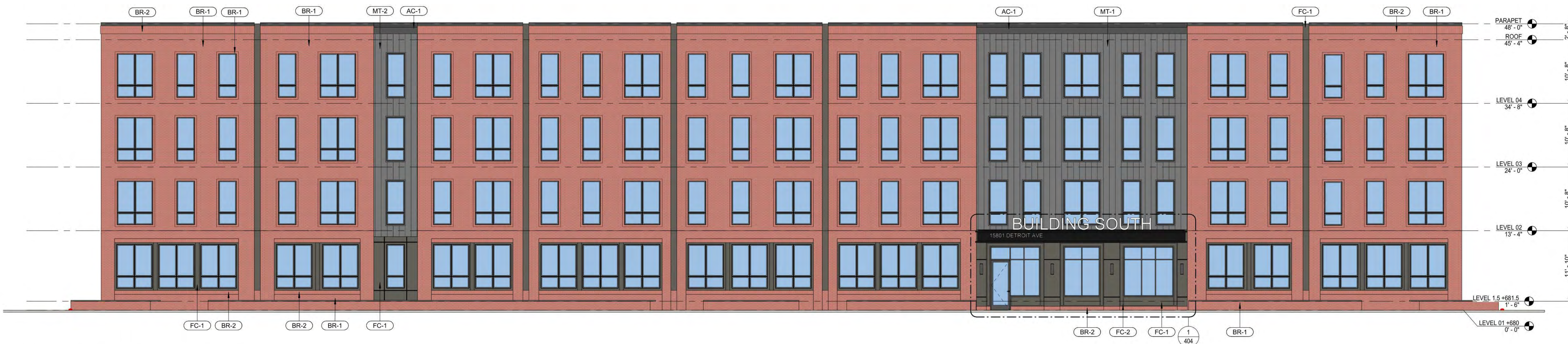
1 BUILDING SOUTH - NORTH ELEVATION SCALE: 1/8" = 1'-0"
