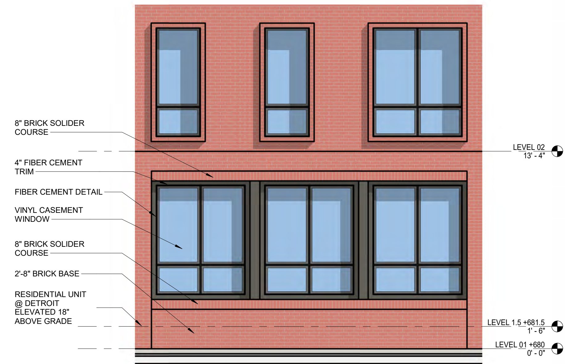
3 TYPICAL RESIDENTIAL WINDOW DESIGN - DETROIT AVE. SCALE: 1/4" = 1'-0"
