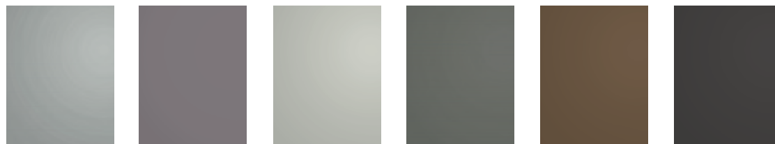
Bright Silver SR:0.55 E:0.85 SRI:64 Rosalind Rose SR:0.32 E:0.88 SRI:34 Champagne Gold SR:0.49 E:0.88 SRI:56 Pewter SR:0.41 E:0.89 SRI:46 Medium Bronze SR:0.15 E:0.89 SRI:12 Dark Bronze SR:0.08 E:0.89 SRI:3
