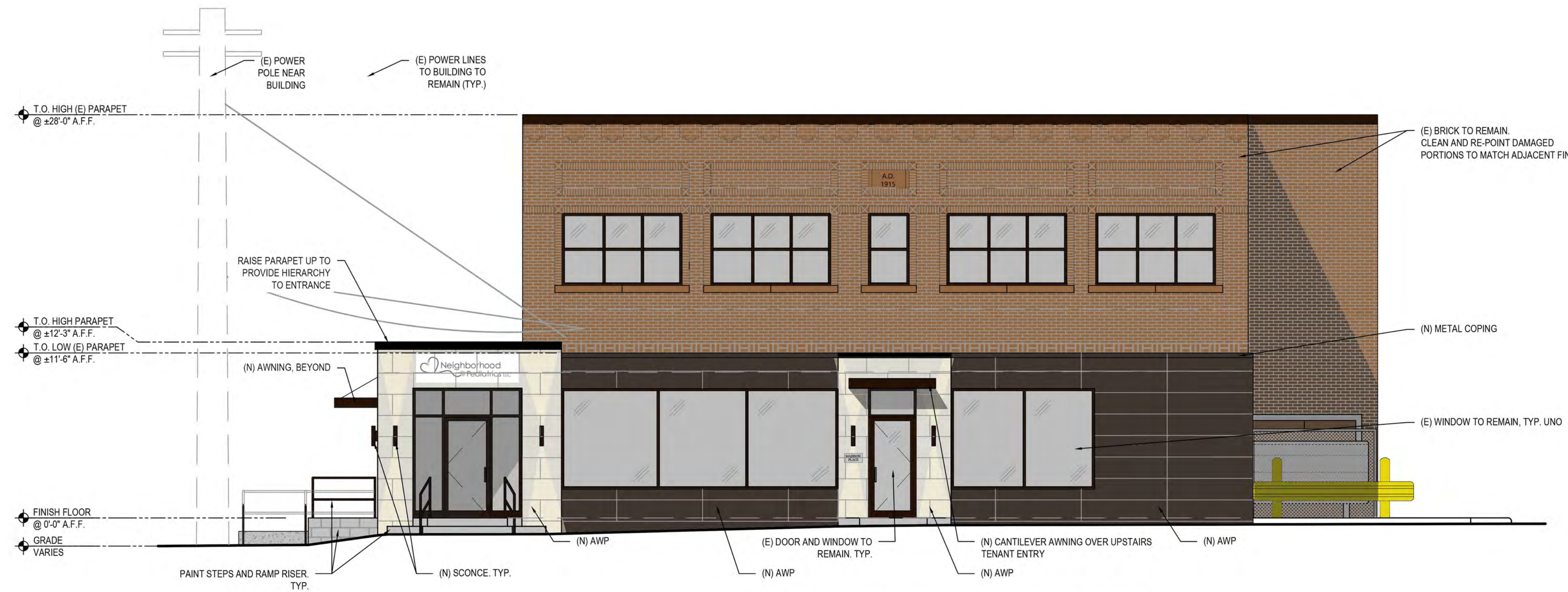
1 SOUTH ELEVATION- MADISON AVENUE SCALE: 3/16" = 1'-0"
