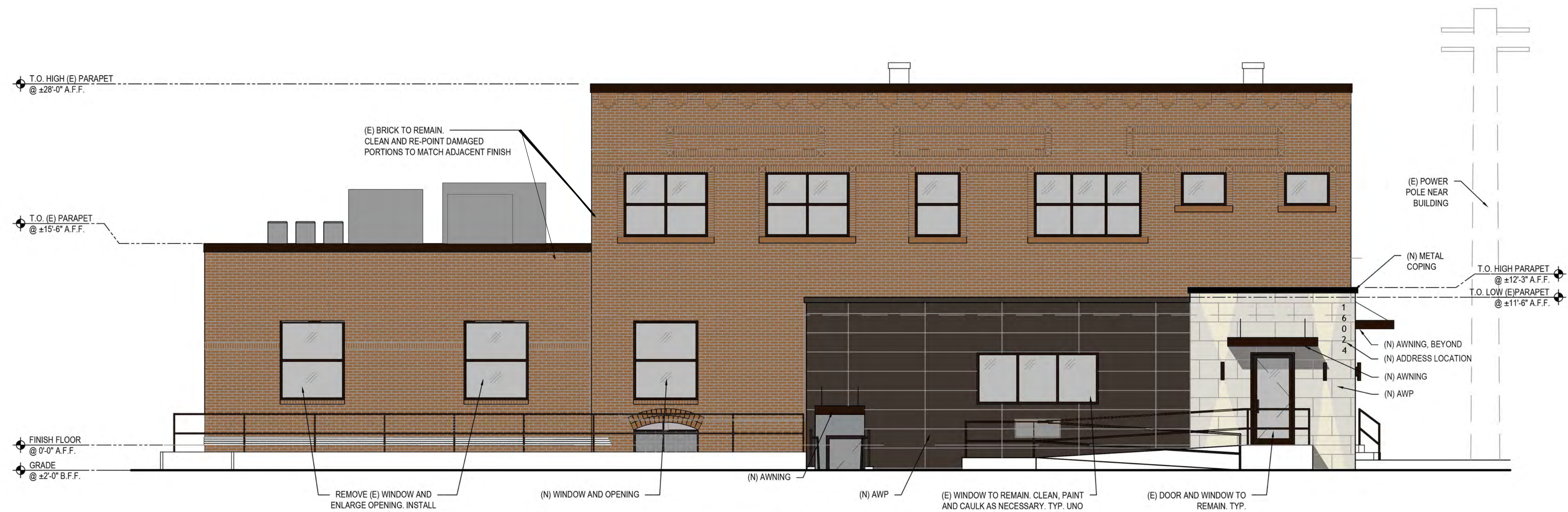
2 WEST ELEVATION - NORTHLAND AVE SCALE: 3/16" = 1'-0"
