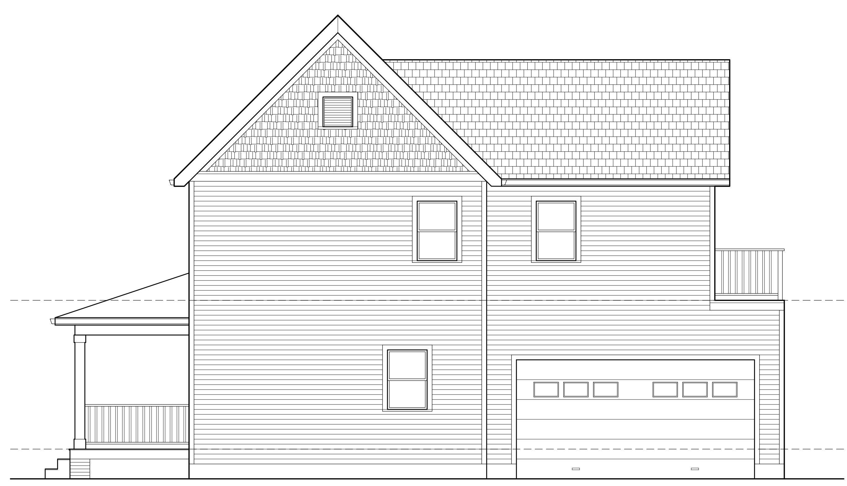
RIGHT SIDE ELEVATION 1/4" = 1'-0" B A1/A2
