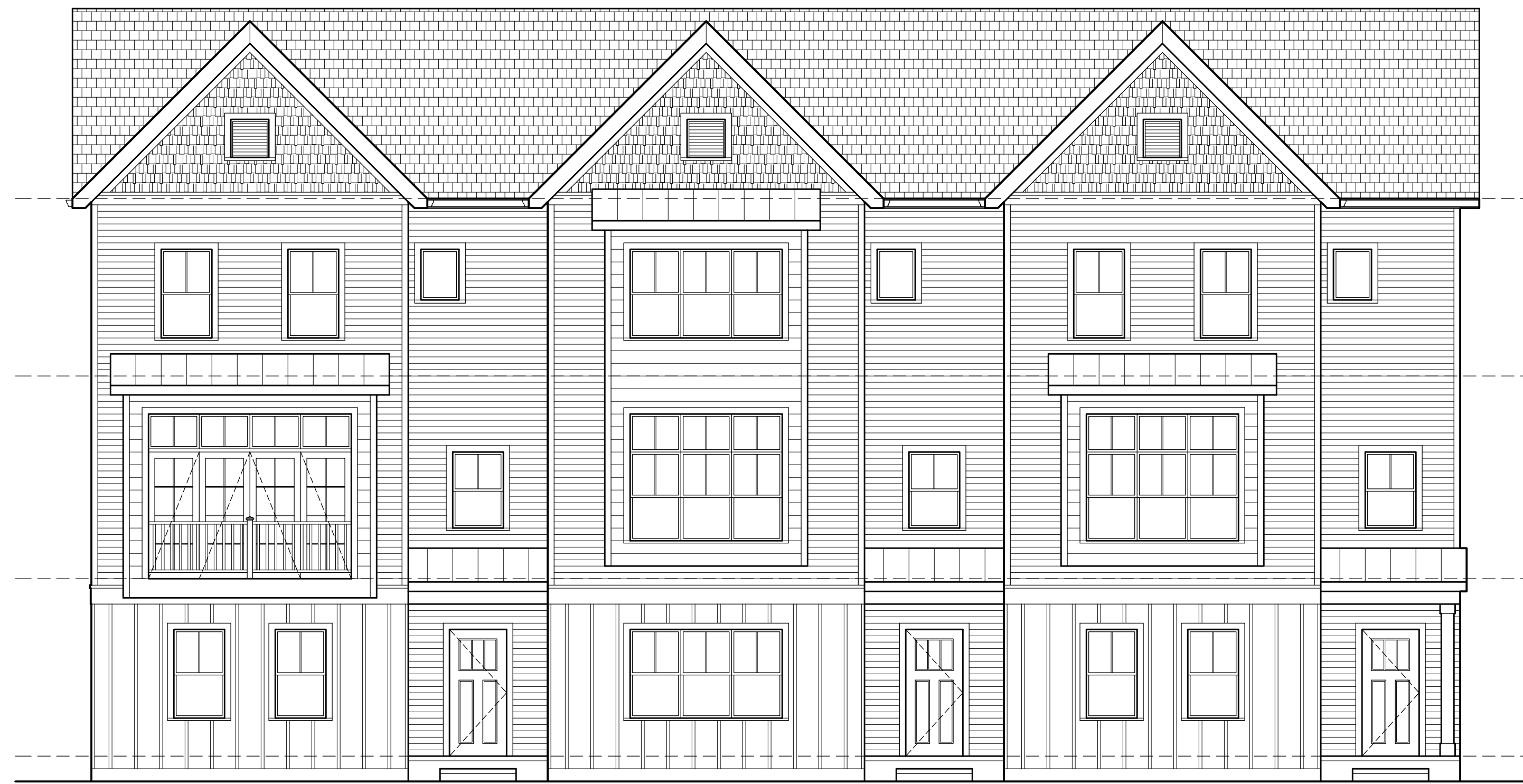
FRONT ELEVATION 1/4" = 1'-0" A
