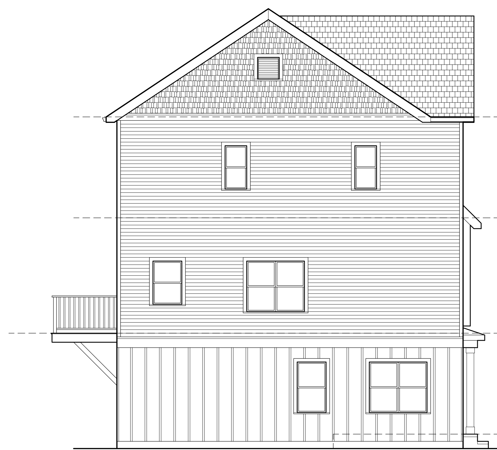
LEFT SIDE ELEVATION 3/16" = 1'-0" B
