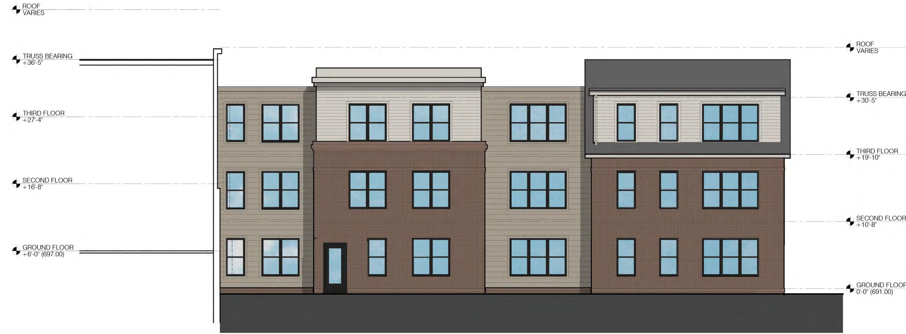
West Courtyard Elevation
